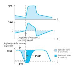
In contrast to the PEEPi measurement in a prolonged expiratory hold manoeuvre, the intrinsic PEEP can also be continuously recorded under spontaneous breathing if the oesophageal pressure measurement catheter is correctly positioned. This enables, for example, a PEEP adjustment with the aim of minimising the intrinsic PEEP.
