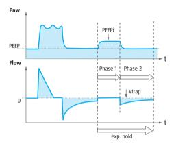
Independent of the adjustable PEEP level, a functional PEEP can also be effective, which is caused by incomplete exhalation.
