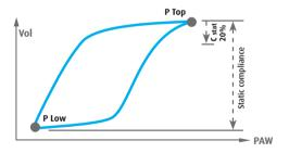
The index C20/C is calculated based on the individual measurements of the PEEPfinder.
